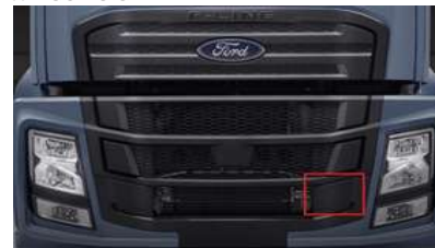
The radar is behind the front grille.
