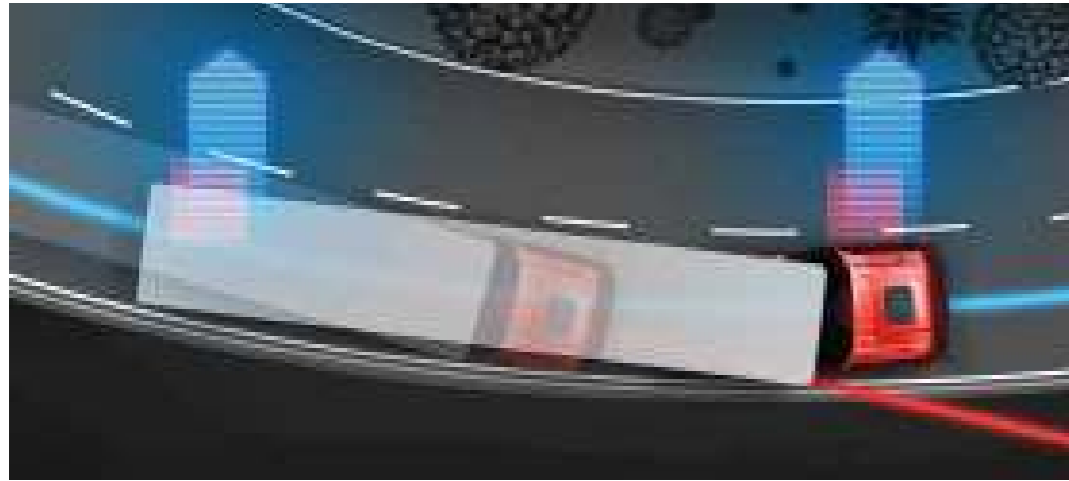
ELECTRONIC STABILITY PROGRAM (ESP) Maintains vehicle balance at different road and climate conditions by interfering with the braking system to prevent the risk of skidding and tipping.
