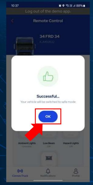
Click the "Safe Mode" button to put your vehicle in safe mode. In this mode, your vehicle's doors will be locked and the windows and lights will be turned off.
