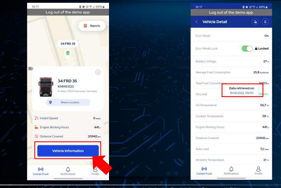
To view your vehicle's data, click on the vehicle icon and click the "Vehicle Information" button. To view the date when the relevant data was last retrieved from the vehicle, you can open the "Last data retrieved" window by clicking on the related data line.
