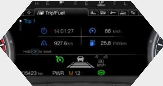
Trip Computer Displays all trip data such as driving distance and average fuel consumption
