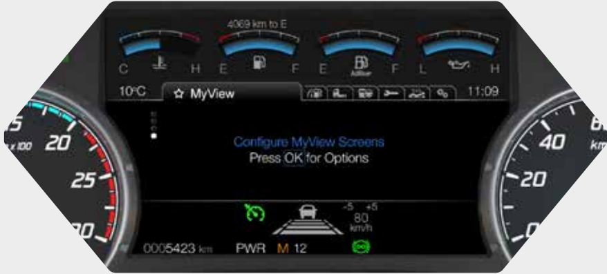
Trip Computer Displays all trip data such as driving distance and average fuel consumption
