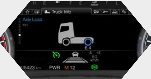
Axle Load Indicator Prevents excessive and incorrect loading by displaying the rear axle load status
