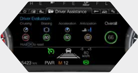
Driver Evaluation Analyses and scores driving style based on criteria such as braking and acceleration during the journey, shares a recommendation screen to improve driving if activated
