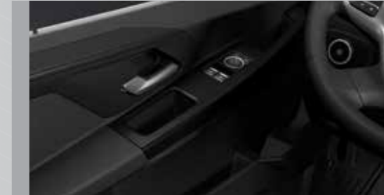
Indoor storage, window and mirror controls
