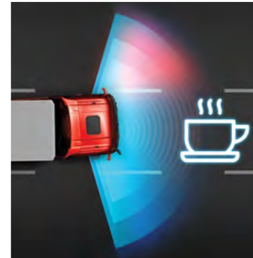
DDAWS - DRIVER ALERT SYSTEM Uses camera-based analysis to detect driver distraction and reduces potential risks with early warnings.
