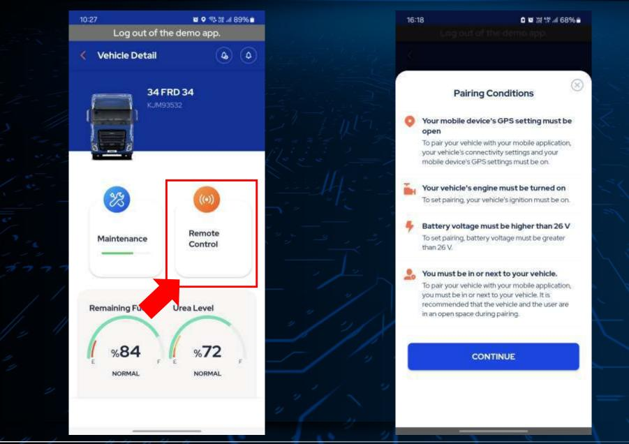
To control your vehicle remotely, click the "Remote Control" button. To control your vehicle remotely, you must first pair the application with your vehicle. If you meet the conditions of the pairing process, the pairing process will be completed successfully. If you do not meet the pairing conditions, you will see the relevant warning on the screen.
