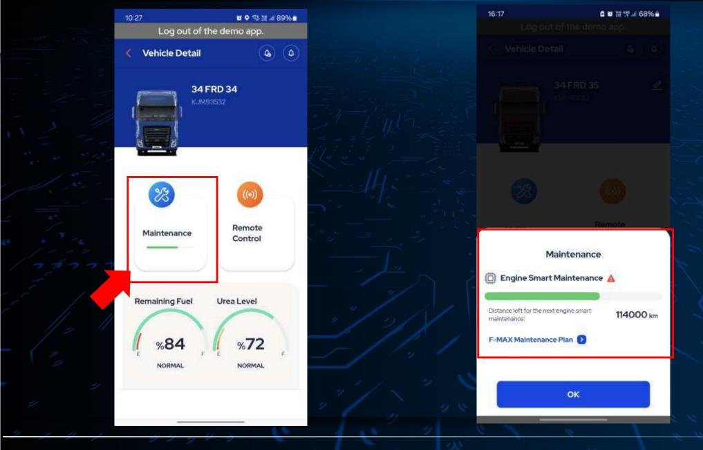
Click the "Maintenance Status" button to view the maintenance status of your vehicle. In the window that opens, you can view the remaining distance to your vehicle's smart maintenance and your maintenance plan.
