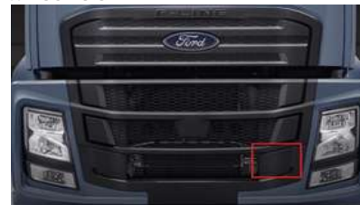
The radar is behind the front grille.
